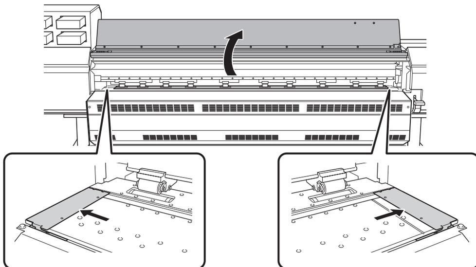
4. (Move to the rear of the printer.) Release the locking mechanisms of the media holders, and then draw them to the left and right ends respectively.
