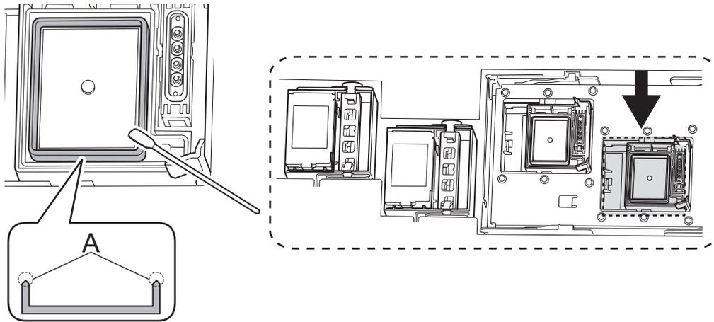
**10.** Use the cleaning stick to wipe off location A (the tip) shown in the following figure in the color ink section.
