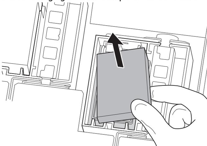
**12. Attach the new flushing pad to the flushing receptacle.**
