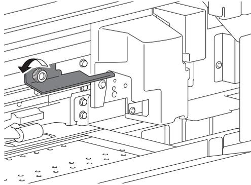
3. Install the retainer at the position indicated in the figure for storage.
