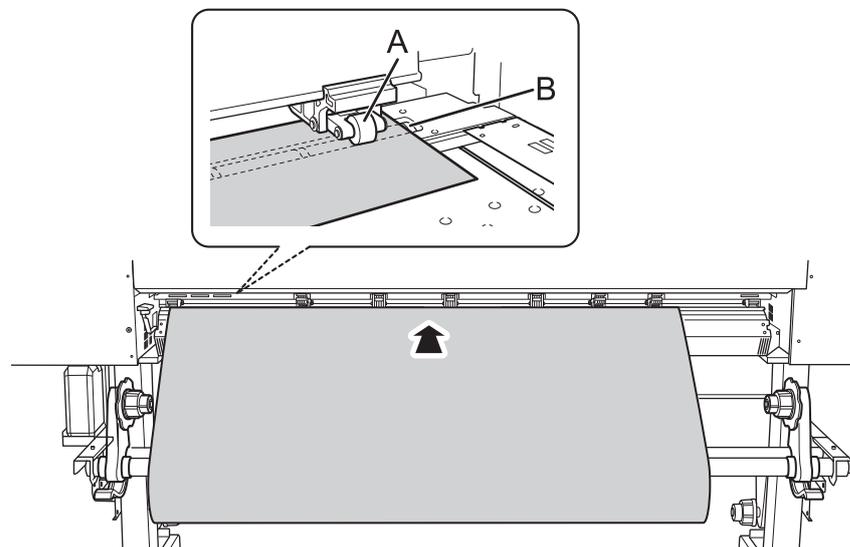
7. (Move to the front of the printer.) Insert the leading edge of the media into the dryer.
