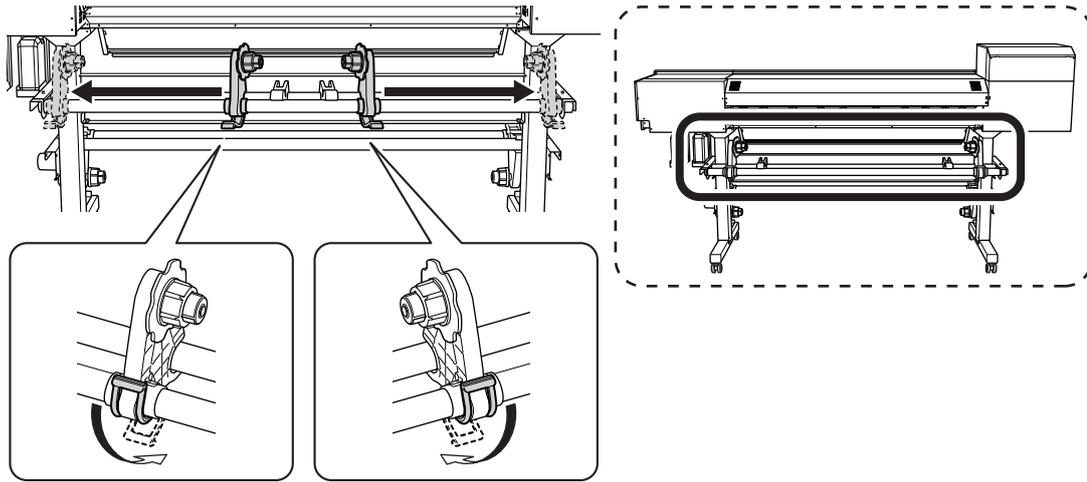
6. From the rear of the printer, pass the leading edge of the media between the pinch rollers (A) and the grit rollers (B).
