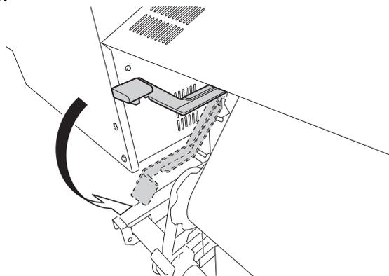
8. (Move to the front of the printer.) Gently hold down the media and raise the loading lever (front).
