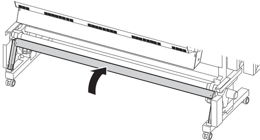
2. Follow the procedure below to load a paper tube on the media holders of the take-up unit.
