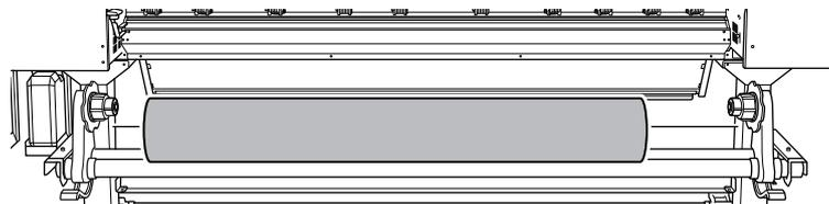
7. Fit the paper tube (core) of the media onto the end cap of the left media holder.
