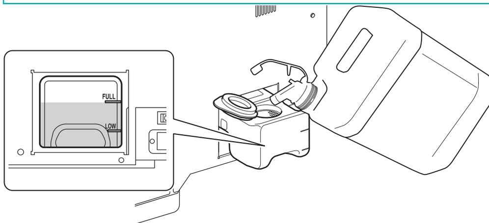
3. Close the lid of the cleaning liquid tank, and then slowly return this tank to its position in the printer.
