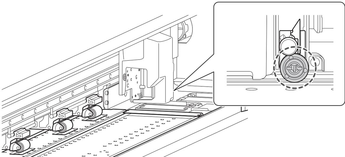
Open the right cover and clean by wiping with a cloth moistened by neutral detergent diluted with water then wrung dry.
