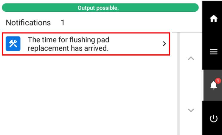
The [Flushing Pad Replacement] screen appears.
