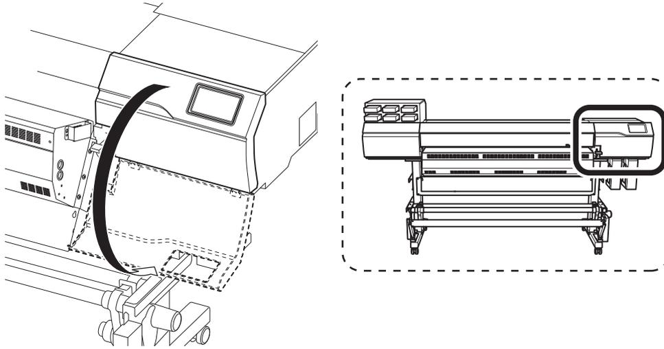
8. Touch the location shown in the figure to discharge any static electricity.
