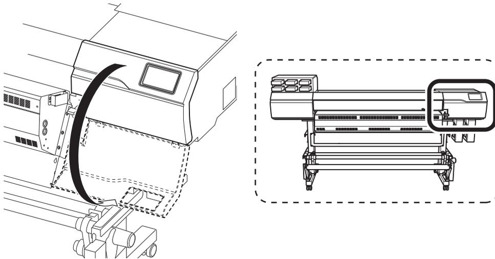
**7. Touch the location shown in the figure to discharge any static electricity.**
