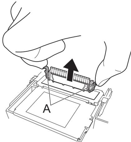
10. Attach the new wiper by inserting it from above.
