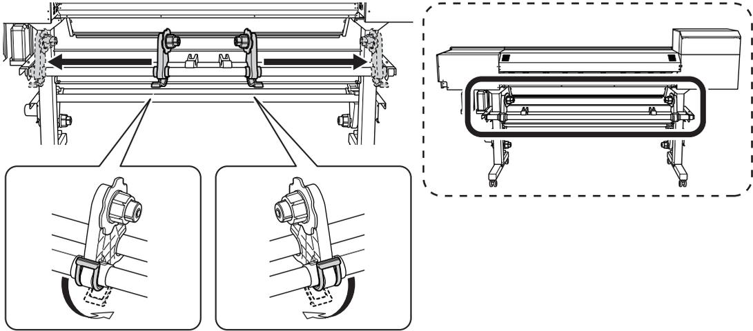
6. Pass the leading edge of the media between the pinch rollers (A) and the grit rollers (B).
