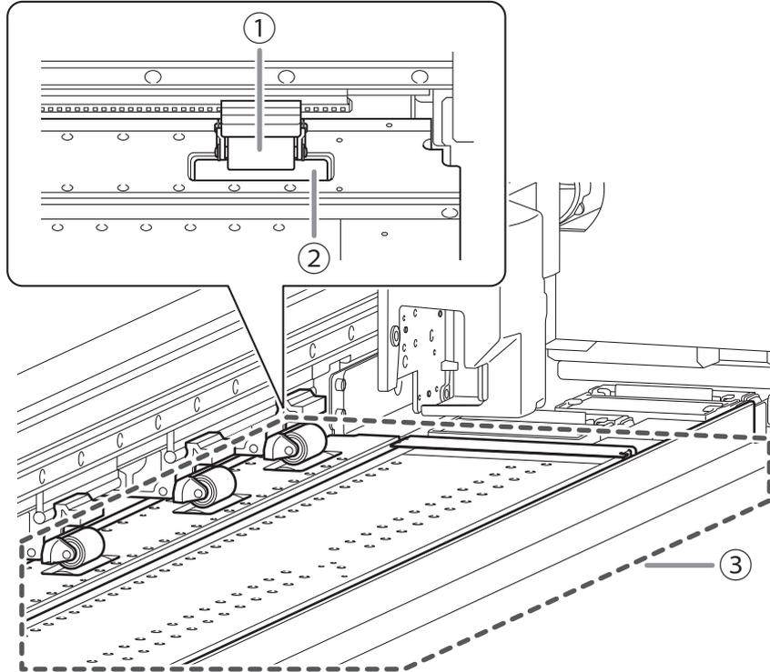
Clean by wiping with a cloth moistened by neutral detergent diluted with water then wrung dry.
