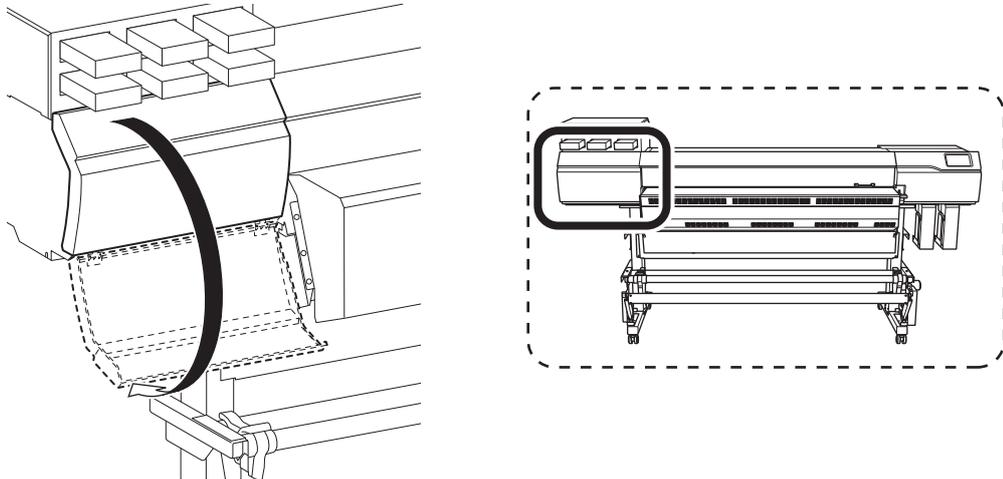
2. Remove the retainer from inside the left cover of the machine.
