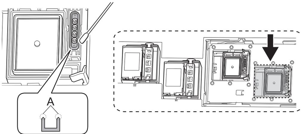
**11.** Use the same cleaning stick to wipe off the flushing frame in the color ink section.
