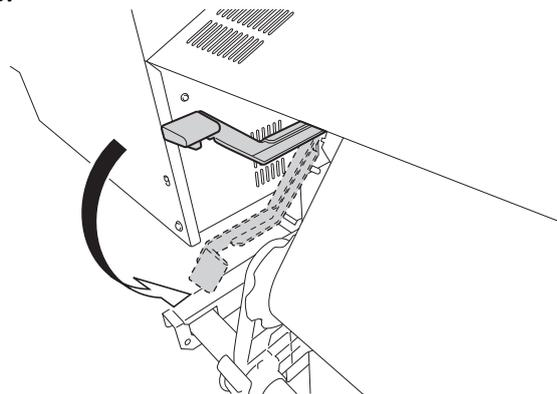
7. (Move to the front of the printer.) Gently hold down the media and raise the loading lever (front).
