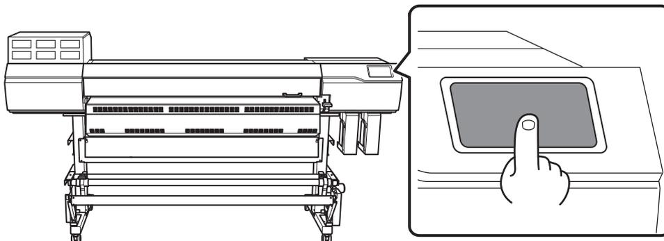
4. When instructions appear on the screen, tap the operation panel again. The power to the operation panel is switched on.
