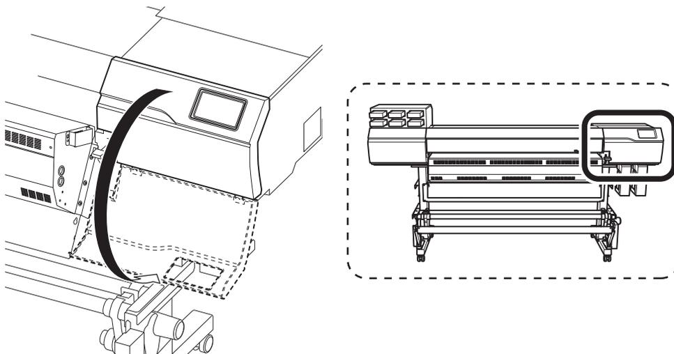
8. Remove the frame to be replaced.
