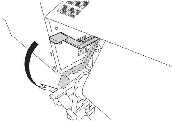
6. (Move to the front of the printer.) Gently hold down the media and raise the loading lever (front). The media is released.
