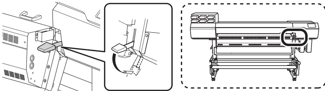
**11. Line up the edges of the media with the centers of the holes of the left and right media clamps.**
