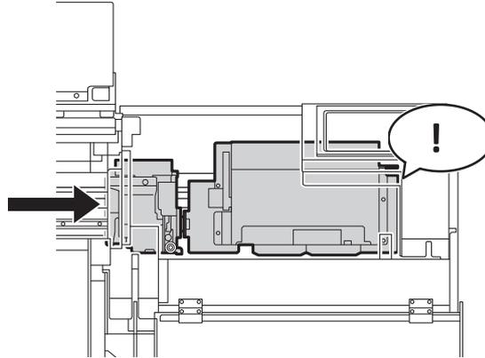
5. Gently apply pressure from the right side to make sure the print-head carriage does not move to the left.
