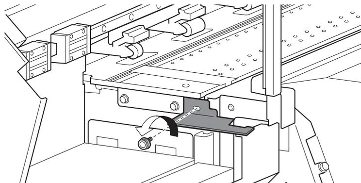
3. Catch the retainer on hole A, and then use the screw to secure the retainer in the position shown in the figure.
