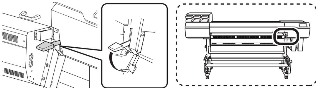
10. Line up the edges of the media with the centers of the holes of the left and right media clamps.
