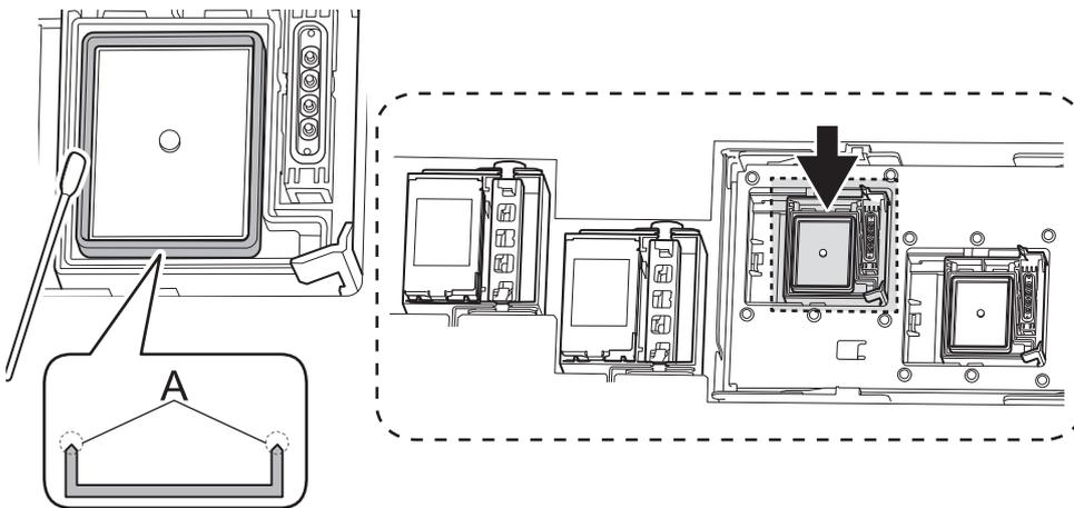
15. Use the cleaning stick to wipe off location A (the tip) shown in the following figure in the optimizer ink section.
