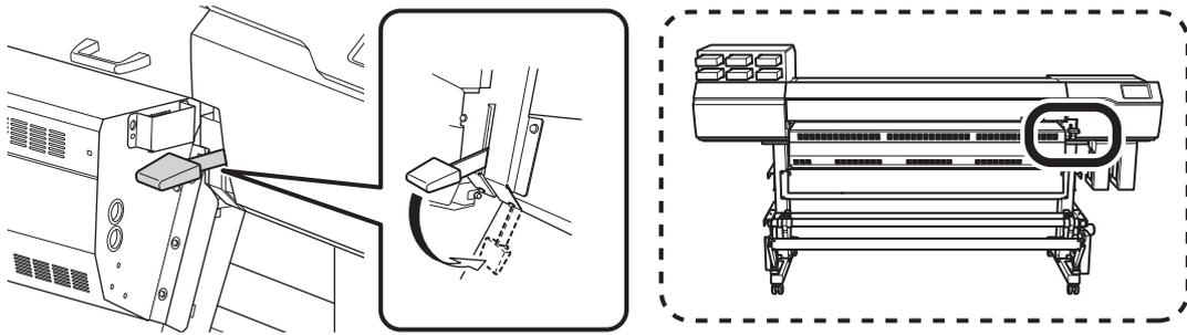
7. Line up the edges of the media with the centers of the holes of the left and right media clamps.
