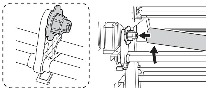
8. Move the right media holder to fit its end cap onto the paper tube (core) of the media.
