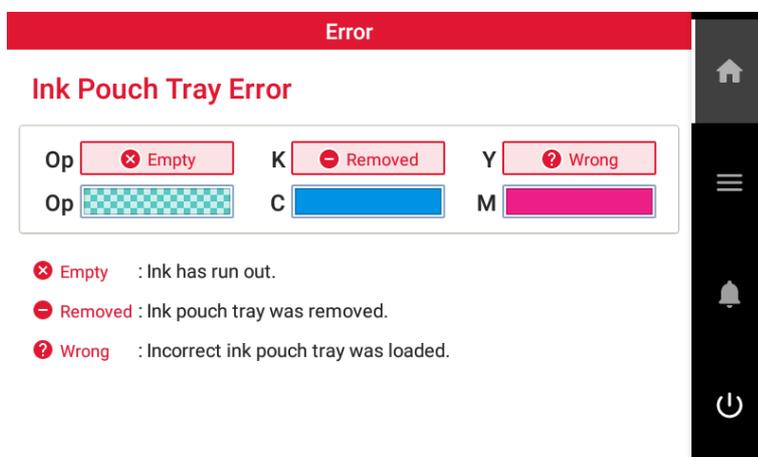
When an [Ink Pouch Tray Error] appears on the display screen, output data cannot be accepted. If there is data that has not yet been output remaining in the machine, output resumes when the error is cleared. If there is unsent data in the computer, output resumes when the data is resent.
