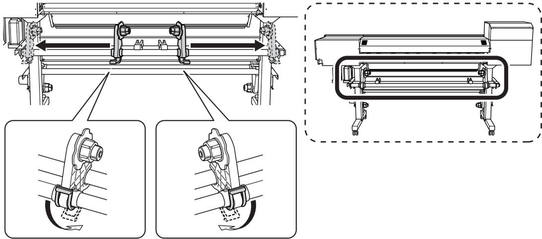
5. Pass the leading edge of the media between the pinch rollers (A) and the grit rollers (B).
