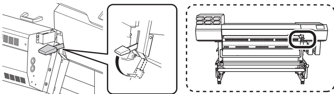
12. Line up the edges of the media with the centers of the holes of the left and right media clamps.
