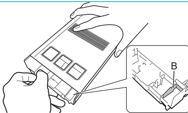
4. Pinch the hook (A) at the tip of the ink pouch, and then remove the ink pouch from the pouch tray.
