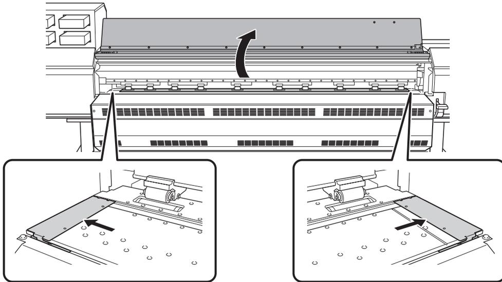
5. Release the locking mechanisms of the media holders, and then draw them to the left and right ends respectively.
