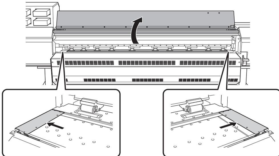
5. (Move to the rear of the printer.) Release the locking mechanisms of the media holders, and then draw them to the left and right ends respectively.
