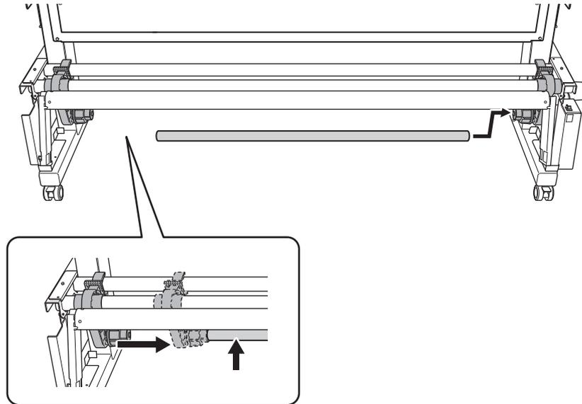
3. Hold down
