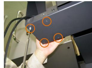
打印开关模块安装螺钉
